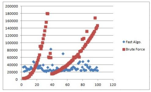
In the chart of runtimes, the x axis is the length of the array input. The y axis is the measured runtime in nanoseconds.
