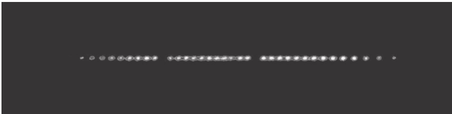
Figure 7.15. Image of fluorescence from about 40 trapped mercury ( ^{199}\text{Hg}^+ ) atomic ions. The ions are spaced by approximately 15 micrometers, and the two apparent gaps are different isotopes of mercury which do not respond to the probe laser. Reprinted courtesy of D. Wineland, at NIST.
