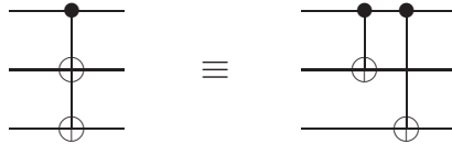
Figure 4.13. Controlled-NOT gate with multiple targets.
