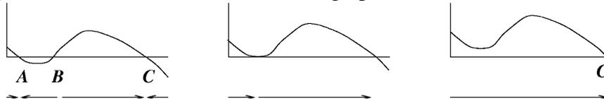
We see that for  $s < s^*$ , there are two sinks (stable steady states), marked  $A$  and  $C$  respectively, as well as a source (unstable steady state), marked  $B$ .
