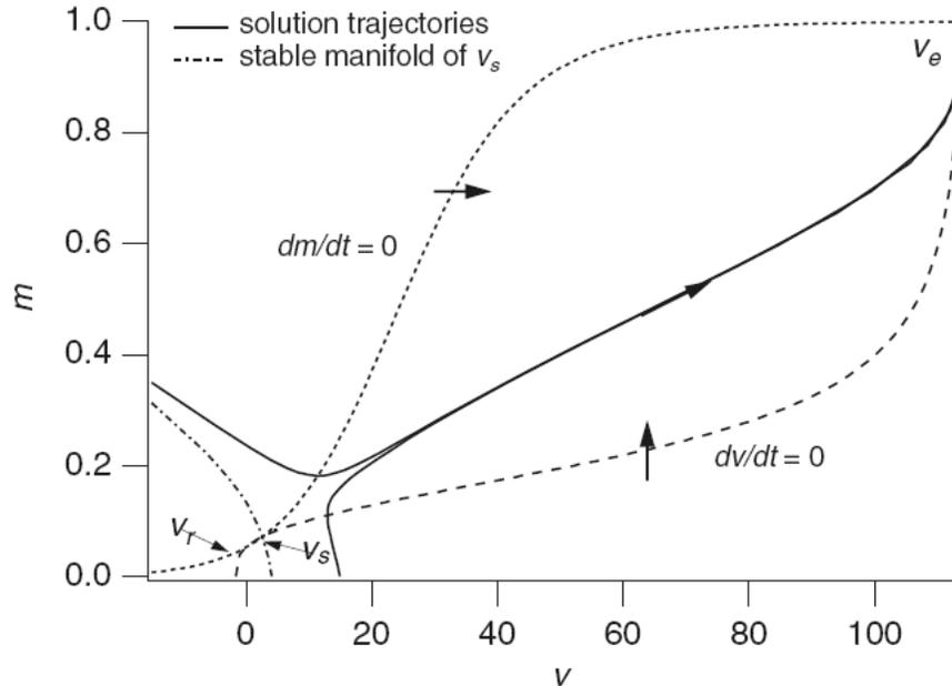
There are two stable steady states:  $v_r$  (“resting”) and  $v_e$  (“excited”), as well as a saddle  $v_s$ . Depending on where the initial voltage (set by a transient current  $I$ ) is relative to a separatrix, as  $t \rightarrow \infty$  trajectories either converge to the “excited” state, or stay near the resting one.
