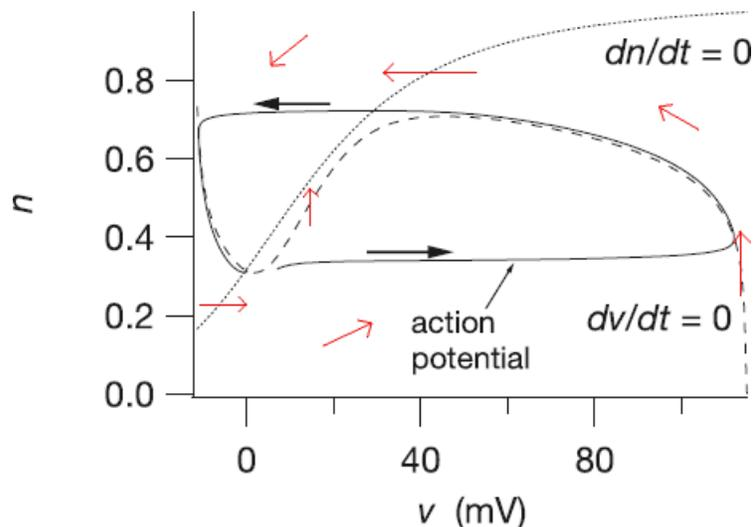
We have fast behaviors on the horizontal direction ( $n = \text{constant}$ ), leading to  $v$  approaching nullclines fast, with a slow drift on  $n$  that then produces, as we saw earlier when studying a somewhat simpler model of excitable behavior, a “spike” of activity.
