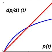
Observe that, for small  $p$ , the formation rate is larger than the degradation rate, while, for large  $p$ , the degradation rate exceeds the formation rate.
