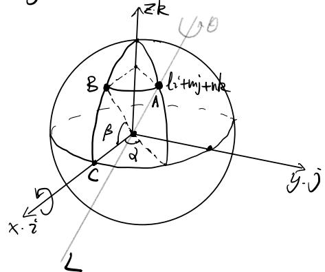
$$P \mapsto f_1(P) = g_2(\beta) \underbrace{g_3(-\alpha)}_{A \rightarrow B} \cdot P \cdot \underbrace{g_3(\alpha)}_{B \rightarrow C}^{-1} g_2(\beta)^{-1} \quad \text{where } g_3(\alpha) = \cos \frac{\alpha}{2} - \sin \frac{\alpha}{2} k$$
