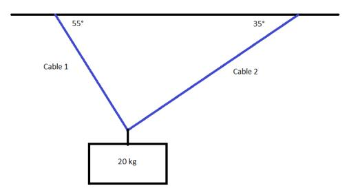
Three forces act at the point where the mass is suspended,  $\vec{F}_1$  along cable 1,  $\vec{F}_2$  along cable 2, and  $f_g = \|\vec{F}_g\| = (20kg)(-9.8m/s^2) = -196N$  which is the force of gravity acting on the mass in the downward direction. Since the block has constant position, its acceleration must be zero and therefore the net force at the point of intersection is zero.
