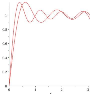
Note that the left endpoint has  $y(0) = 0$  for both curves, but the right endpoint has different values of  $y(\pi)$ , although  $y(\pi) + y'(\pi) = 0$  for both curves. This is expected for this case since each term of the eigenfunction expansion has  $y(\pi) \neq 0$
