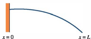
(b) Cantilever beam: embedded at the left end, free at the right end
