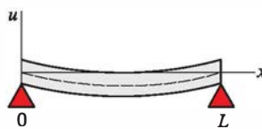
FIGURE 13.4.9 Simply supported beam in Problem 23
