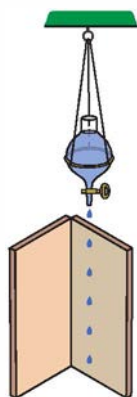
FIGURE 1.3.1 Da Vinci's apparatus for determining the speed of falling body
