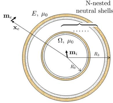
Figure 4. A shield of  $N$ -nested neutral shells.
