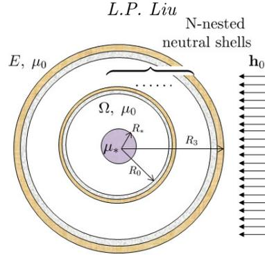
Figure 5. Cloaking effect of a shield of nested neutral shells.
