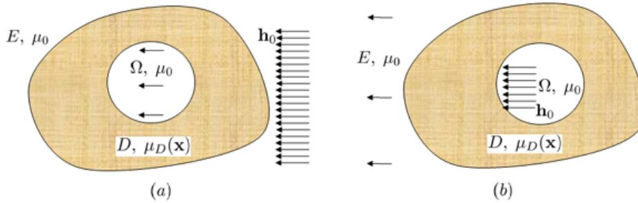
Figure 1. (a) A shield for field expelling; (b) A shield for field confinement.
