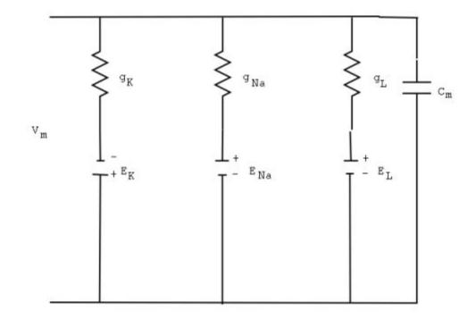
Note that each ion channel is viewed as a resistor, with voltage drop  $V - V_i$  and conductance  $g_i$ , for i = Na, K, L. Recall that resistance and conductance are inverses of one another, as  $C = \frac{1}{R}$ . Furthermore, writing the circuit in parallel assumes *linearity*, which is an **assumption**,
